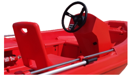
STEERING CONSOLE WITH A WHEEL, GEAR, STEERING SYSTEM AND LIGHTER SOCKET
