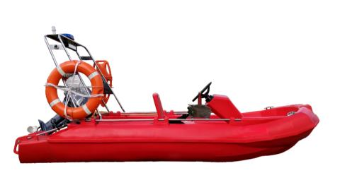
AS A STANDARD FEATURE, THE BOAT'S TRANSOM IS ADAPTED TO L-SHAFT ENGINES. OPTIONALLY, TRANSOM CAN BE ADJUSTED TO THE S-SHAFT ENGINES FOR TILLER ENGINES.
